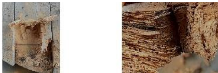
Figure 4: A) Wood dust. B) Aesthetic qualities of borer infestations. (Source: Graham, 2022)
