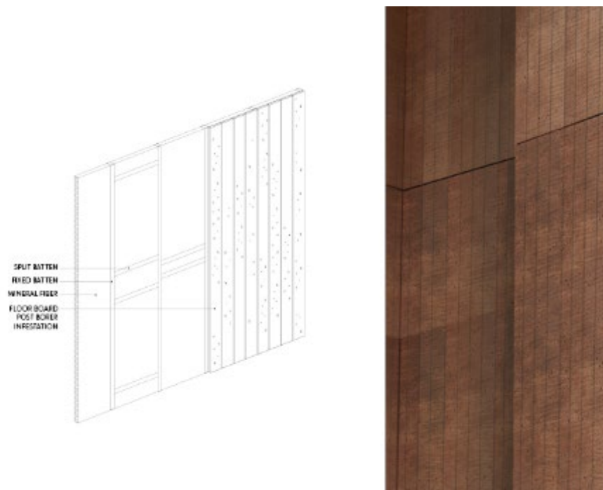
Figure 2: Conceptual application of reused borer timber as acoustic panels. (Source: Graham, 2022)
